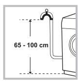
Connect the drain hose, without bending it, to a draining duct or a wall drain situated between 65 and 100 cm from the floor;
